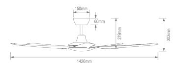
Note: Do NOT install on a raked or sloped ceiling without the use of the optional 38° Ceiling Kit, as this will damage the receiver housed in the canopy.
